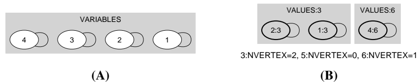
Figure 5.353: Initial and final graph of the global_cardinality constraint
