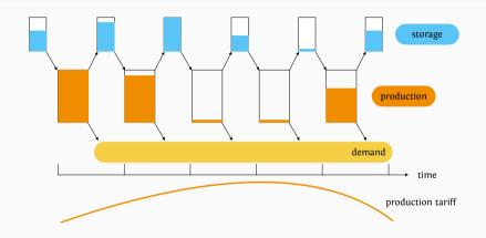
decide on operation and storage levels to meet demand, capacity, and flow conservation on all periods and minimize the total operation cost (**load shifting**)
